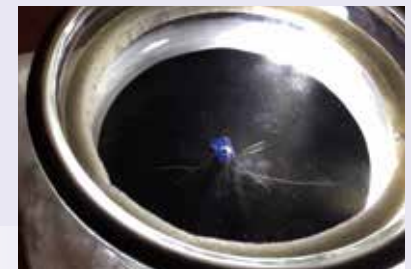
霧箱による放射線源(ユークセン石)から放射状に出るα線の飛跡の観察 A cloud chamber helps visualize the trajectory of alpha rays that are emitted radially from a radiation source (euxenite).
